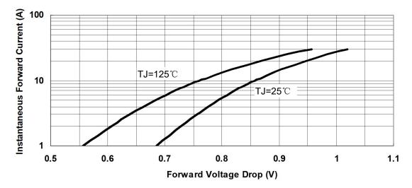
Fig.3-Typical Instantaneous Forward Voltage Characteristics
